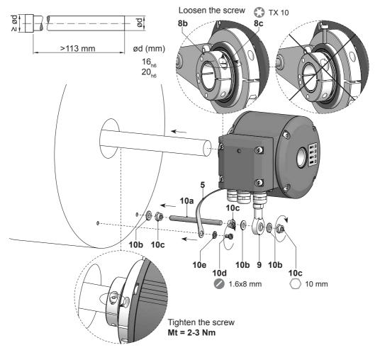
The encoder must be mounted with cable connection facing downward and not exposed to water.
