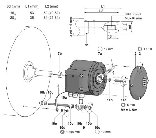
The encoder must be mounted with cable connection facing downward and not exposed to water.
