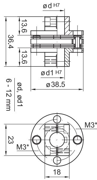
\* max. tightening torque  $M_t = 50 \text{ Ncm}$
