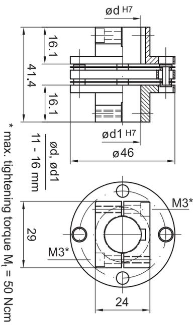
\* max. tightening torque  $M_t = 50$  Ncm
