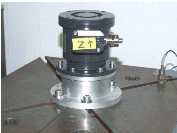
picture 11 Incremental Encoder POG 10 on the shock table with acceleration sensor during shock test in Z-axis, positive direction
