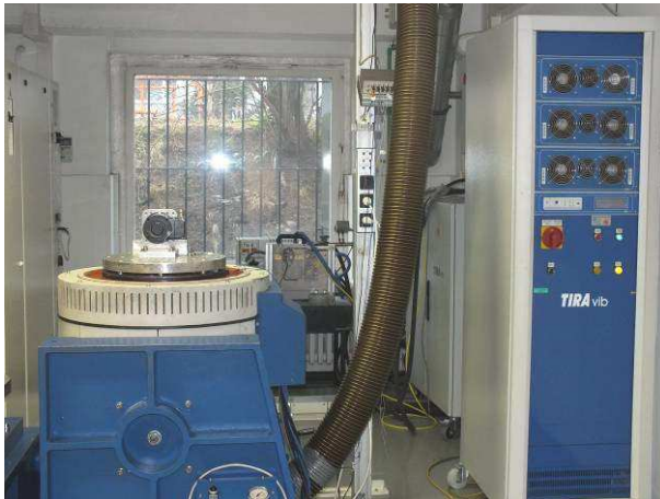
picture 1 Incremental Encoder POG 10 on the vibration test device during vibration test in X-axis
