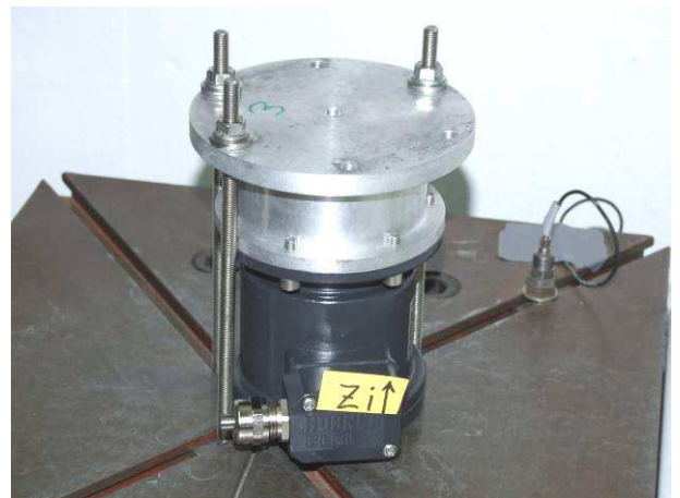
picture 12 Incremental Encoder POG 10 on the shock table with acceleration sensor during shock test in Z-axis, negative direction
