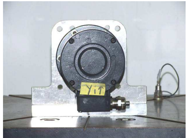
picture 10 Incremental Encoder POG 10 on the shock table with acceleration sensor during shock test in Y-axis, negative direction
