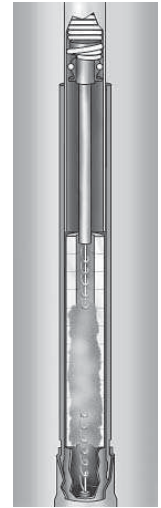
Vapor quenches arc at first current zero
