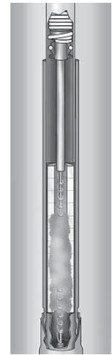
Vapor quenches arc at first current zero
