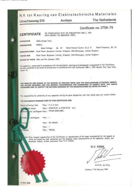
This certificate refers to SFQDJ 36kV fuse links, which are electrically identical to the new T range, other than the fuses are sealed for outdoor use, have a brown ceramic body and use a 50N striker.
