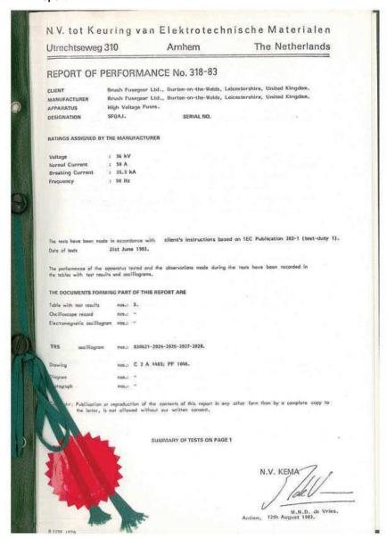
This certificate refers to SFQAJ 36kV fuse links, which are electrically identical to the new T range, other than the fuses are sealed for outdoor use, have a brown ceramic body and use a 50N striker.
