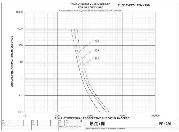
Time current curve - Fuse types TDM/THM/TFM
