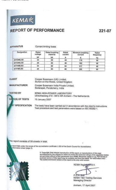
This report of performance details 24kV DIN-rated fuse links tested in accordance with IEC 60282-1:2005 to demonstrate correct operation on a 25kV system.
