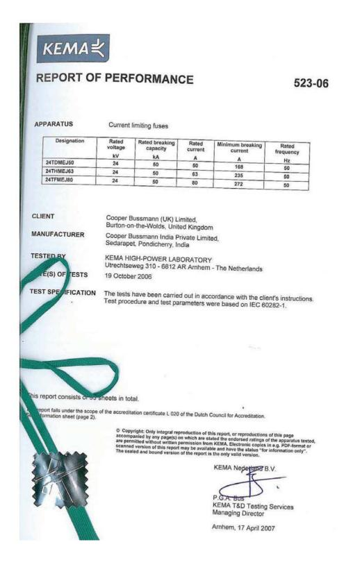
This report of performance details 24kV DIN-rated fuse links tested in accordance with IEC 60282-1:2005 to demonstrate correct operation on a 12kV system.
