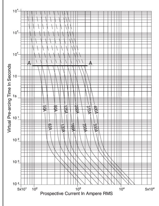
The partial dotted curves are for fuses designed to give part range protection (aR protection). Loading or operation above the curve indicated at A on the curves must in general be avoided. Please see technical guidance 170K...
