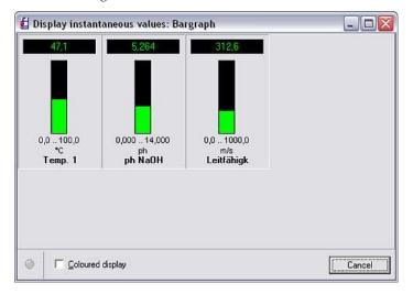
The bar graphs can either be displayed in green or in multiple colors. For multicolored display, select the command **Colored display**.
