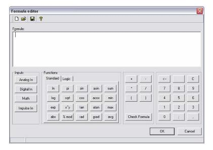
A formula with up to 200 characters can be created with this editor. Once the formula is finished, the **Check formula** function can be used to check whether the formula entered is correct. If the test is positive, the editor can be closed with **OK** and the formula entered is accepted.
