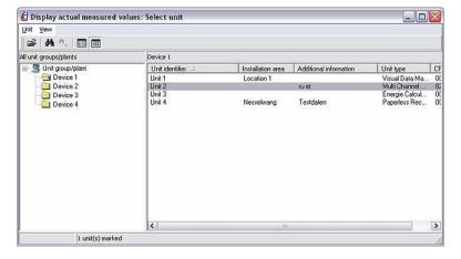
Select a unit from the list of units. The program establishes a connection to the selected unit when you double-click the unit or select  $Unit \rightarrow Open unit$ .
