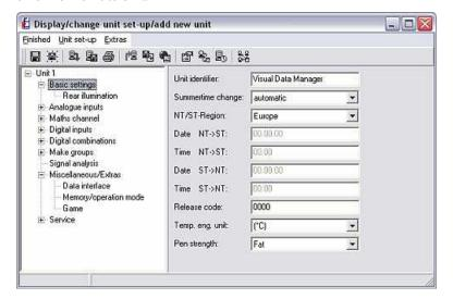
If you want to view or modify the current settings, select the option in question from the list on the left. The settings already made then appear on the right-hand side of the screen. These settings can now be modified. In the text fields, either enter the new values or select a new setting from the drop-down menus.
