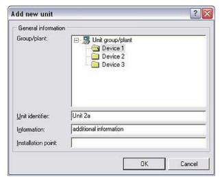
As when creating a new unit (see Section 3.2.4), you can use the imported data for a new unit. To do so, select the **Group/plant** where the unit should be saved. You also have to give the unit a new name in the **Unit identifier** text field.
