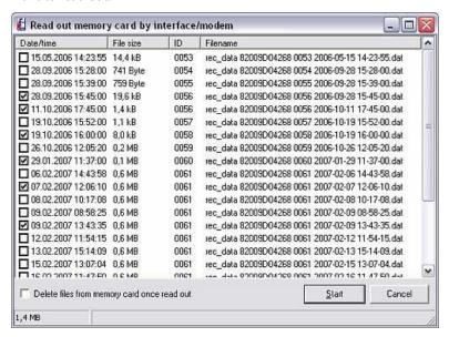
You can read out just one file or all the files from the memory card. You can also choose whether the files should be deleted from the memory card once read out.
