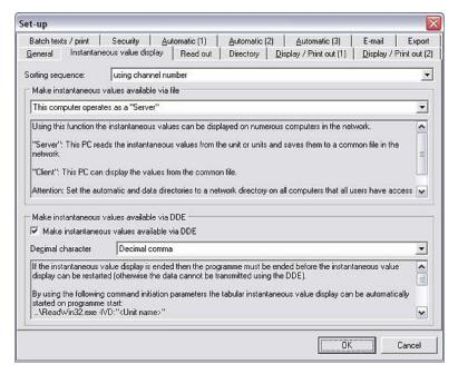
In the **Sorting sequence** field, specify whether the system should sort **Using the channel name** or **Using the channel number**.
