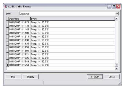
In the **Filter** drop-down menu, you can filter the list based on certain criteria or message texts, or you can display all the events of the time range. The current audit trail can be printed out with **Print**.
