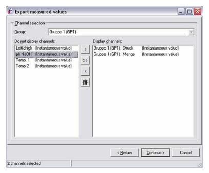
To do so, select the channels required in the field on the left and click the '>' arrow symbol to move the channels to the **Display channels** field. You can also click the double-arrow symbol '>>' to move all the available channels at once. In addition, you can use the back-arrow symbol '<' to move channels back to the **Do not display channels** field.
