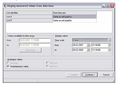
Pressing **Continue** > to confirm opens a screen where you can select the channels that should be displayed. A maximum of 40 channels can be displayed.
