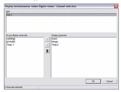
The screen is split into three fields. The units you have selected are displayed in the top field. Selecting a unit causes the unit's active channels to be displayed in the lower left-hand field. Channels can now be selected and moved to the field on the right.
