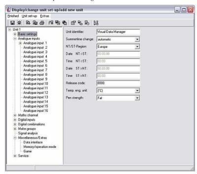
Once you have made the settings, you can send them to the device via the **Send setup to unit** command in the **Finished** menu if this device is connected to the PC.
