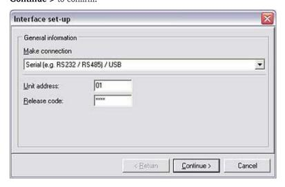
Then enter the appropriate **Interface parameters** and press **OK** to confirm. The connection is made to the unit and the **Service: Unit details** screen appears.
