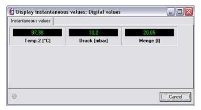
Instantaneous measured values are shown in green. The channel name is marked red if the limit value is violated which means an error can be detected quickly.
