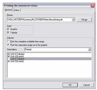
In the **General** tab you can select the printer and type (i.e. graphic and/or table) and you can select the time range, orientation and tables in the **Tabular** field.
