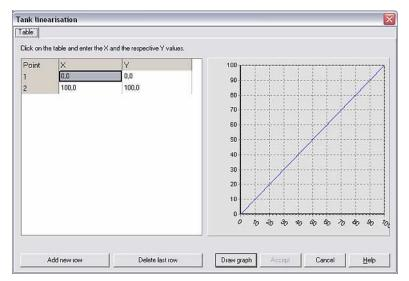
Here, you can **Add a new row** or **Delete the last row**. Double-click the numerical values in the table to change the values. You can display the numerical values with the **Draw graph** command. The **Help** option provides you with detailed help on the linearization table.
