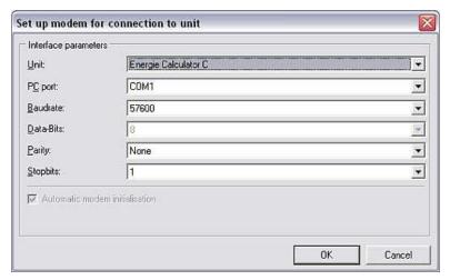
In this dialog box, configure the interface parameters set in the unit and the initialization string for your modem. Activate or deactivate the checkbox to choose whether modem initialization should be automatic or selected from the dropdown menu. After confirming with OK, the modem is configured for use at the unit
