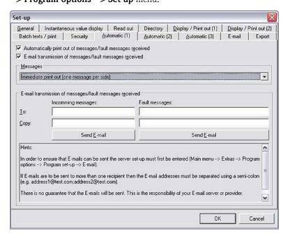
In the screen, select whether incoming (fault) messages should be printed out automatically or forwarded by e-mail. For this purpose, you have to use the text field to enter the target e-mail address where the error reports should be sent.
