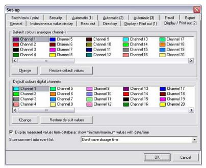
Here, you can also choose whether the minimum and maximum values, and the related date/time, should be shown when displaying measured values from the database. The storage time can be saved with comments in the event list or not.
