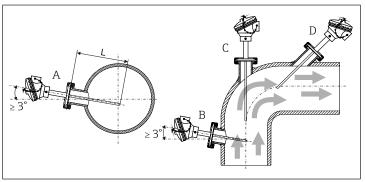
A - B: In pipes with a small cross section the sensor tip should reach or extend slightly past the center line of the pipe (= L). Installation with minimal 3° inclination because of self draining.
