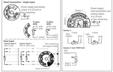
Terminal block mounted (insert with 3" flying leads)
