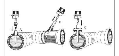
Examples of spring loaded insert installation.
