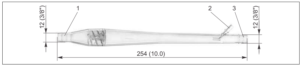
Air trap, dimensions in mm (inch)
