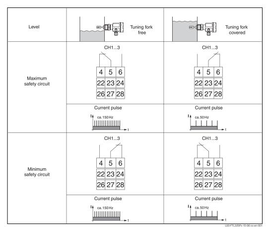
Function of the level limit signal and the current pulse dependent on level and fail-safe circuit.
