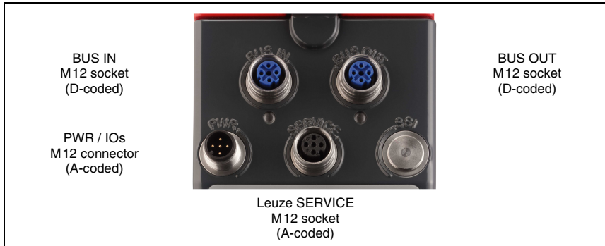
Figure 7.1: Connections of the AMS 358 i
