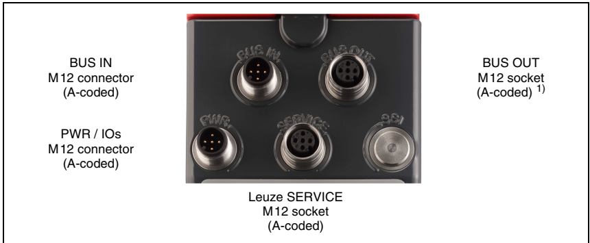
Figure 7.1: Connections of the AMS 355 i
