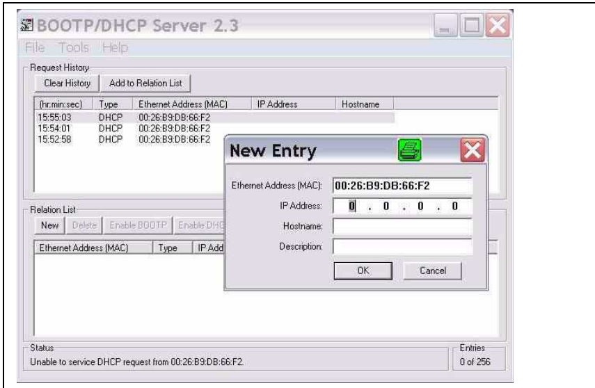
Figure 3.1: Manually setting the IP address
