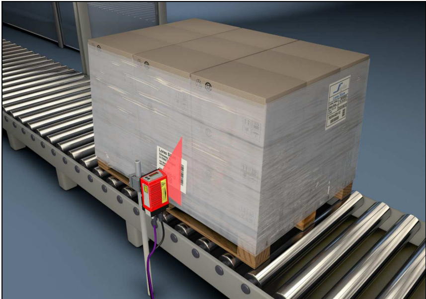
Figure 4.8: Deflection principle for the line scanner
