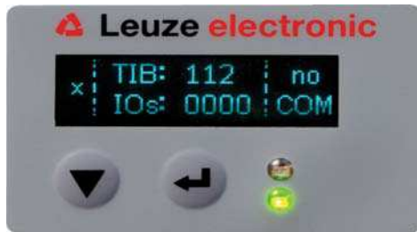
Figure 3.3: OLED display on the receiver
