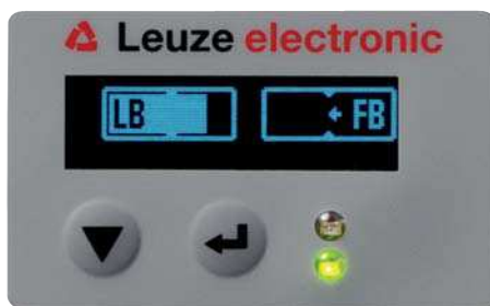
Figure 8.1: Example: display showing an incorrectly aligned light curtain
