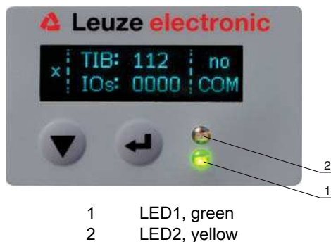
Figure 3.2: LED indicators on the receiver
