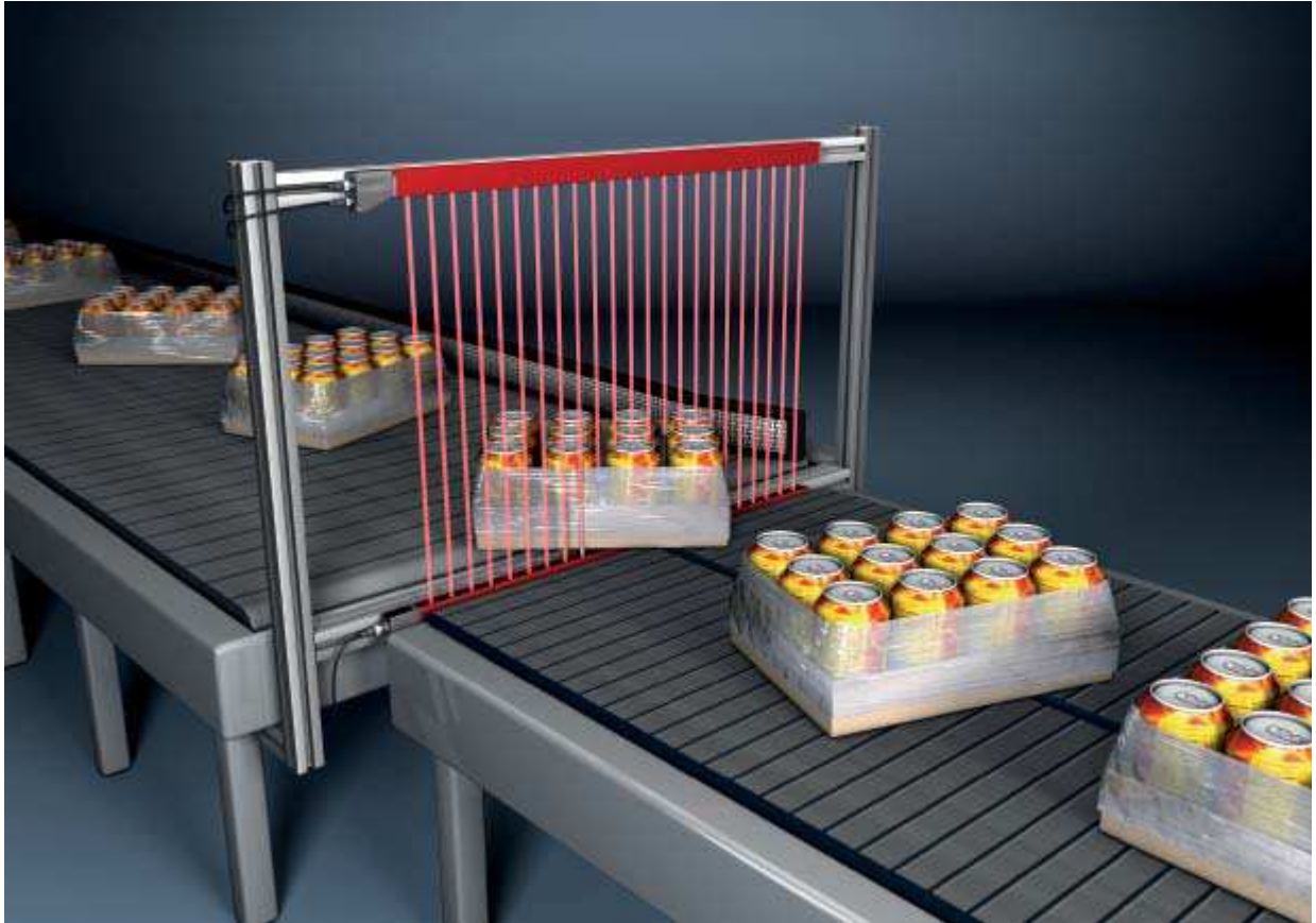
Figure 5.3: Width measurement, orientation detection
