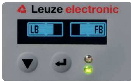
Figure 8.2: Display showing an optimally aligned light curtain
