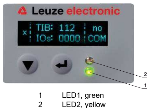
Figure 3.2: LED indicators on the receiver
