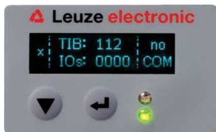
Figure 3.6: Function buttons on the receiver
