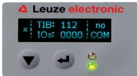
Figure 3.3: OLED display on the receiver
