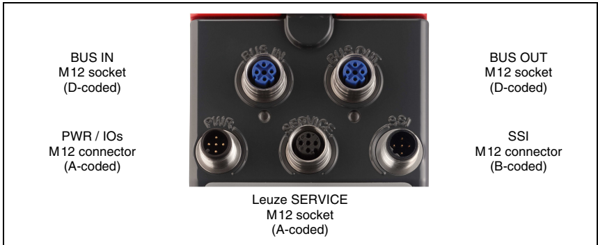
Figure 7.1: Connections of the AMS 348 i SSI
