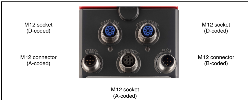
Figure 9.4: Connections of the AMS 348 i
