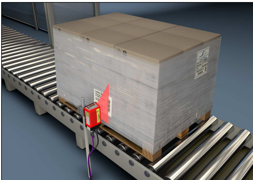
Figure 4.8: Deflection principle for the line scanner
