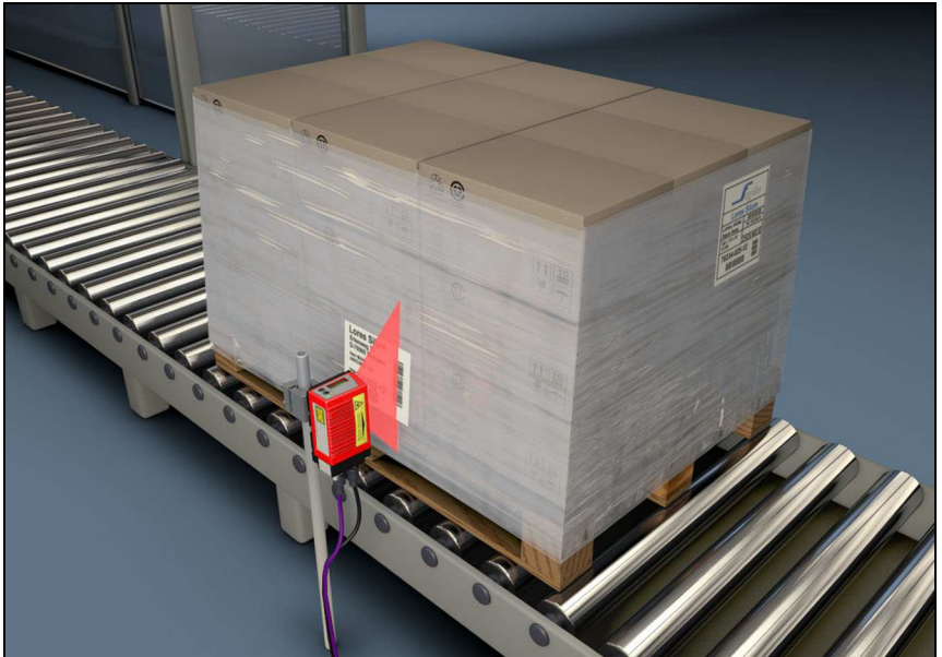
Figure 4.8: Deflection principle for the line scanner
