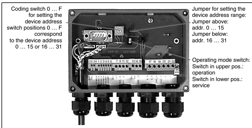
Figure 7.1: Configuration elements in the MA 2
