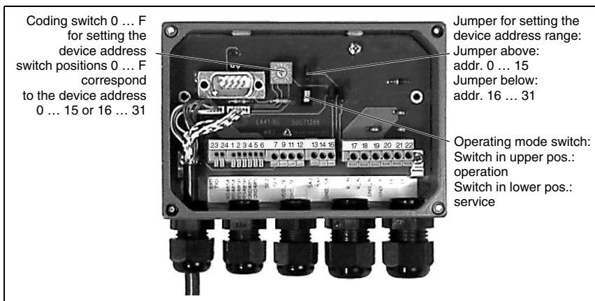
Figure 7.1: Configuration elements in the MA 2
