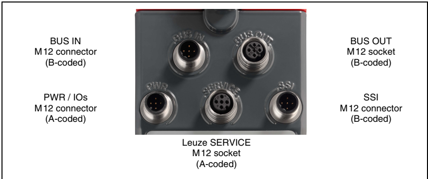
Figure 7.1: Connections of the AMS 304 i
