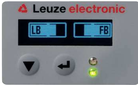
Figure 8.2: Display showing an optimally aligned light curtain
