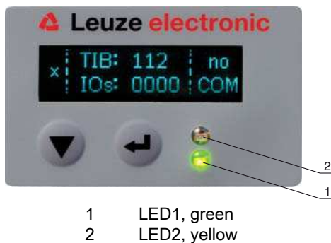
Figure 3.2: LED indicators on the receiver
