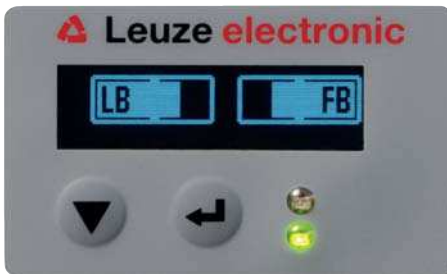
Figure 8.4: Display after successful teach
