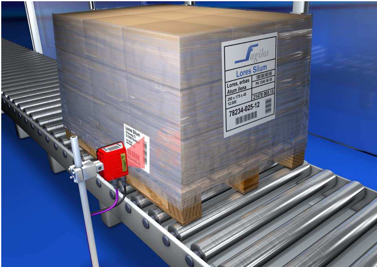
Figure 5.1: Deflection principle for the line scanner
