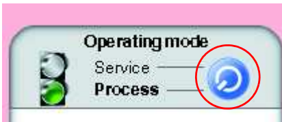
Figure 3.2: Changing the operating mode by means of a button or by selecting a menu item
