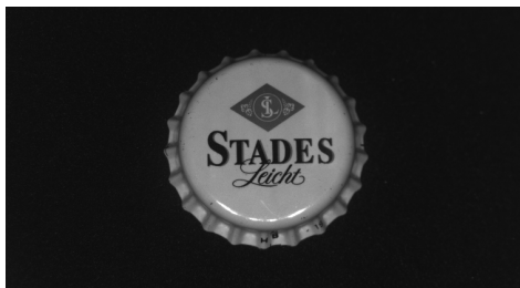
Figure 4.36: Inclined camera alignment with only three illumination quadrants active (reflected quadrant is off) - nearly all reflections in the image are suppressed
