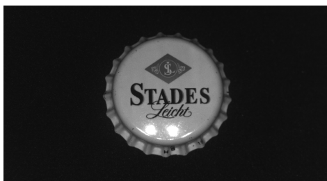
Figure 4.35: Inclined camera alignment with all four illumination quadrants active - better, but reflections still visible in one quadrant
