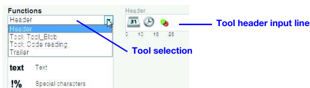
Figure 3.27: Tool selection for the output
