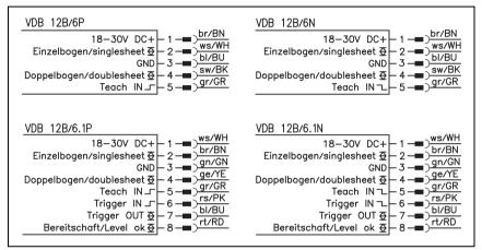
Figure 6.1: Connection diagrams VDB 12 B...
