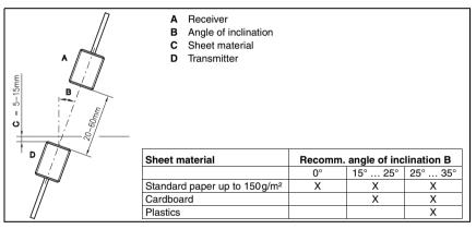
Figure 5.1: Mounting the transmitter and receiver
