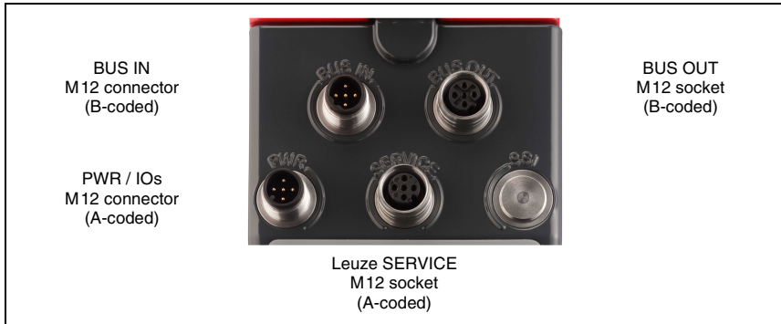
Figure 7.1: Connections of the AMS 301 i
