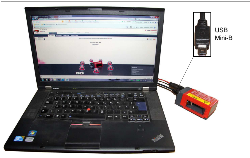
Figure 9.1: Connecting the SERVICE USB interface
