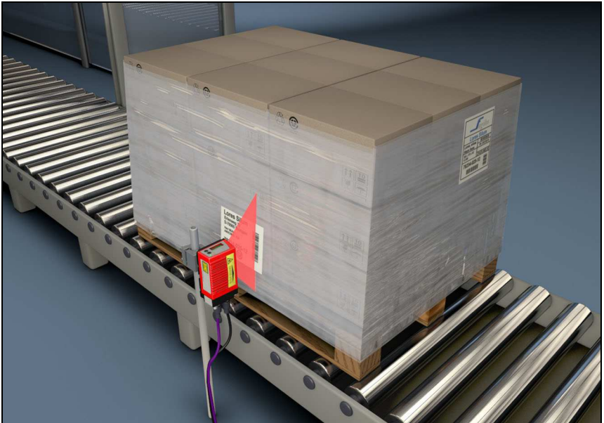
Figure 4.8: Deflection principle for the line scanner
