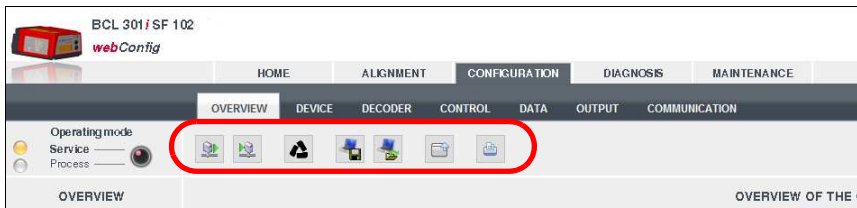
Figure 10.1: Storing configuration data in the webConfig tool
