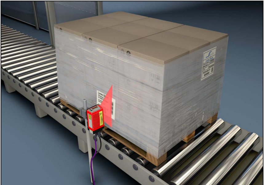
Figure 4.8: Deflection principle for the line scanner
