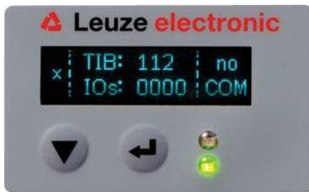
Figure 8.3: Display showing the process mode state of the light curtain
