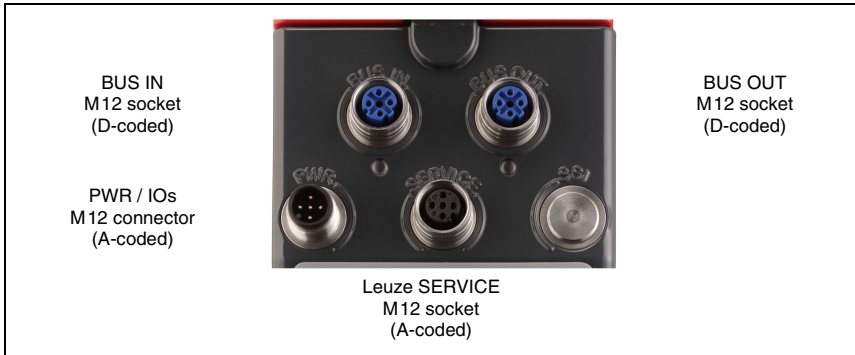
Figure 7.1: Connections of the AMS 308 i
