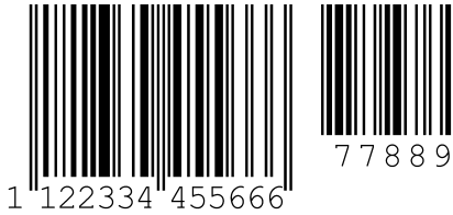
Figure 17.8: Code type: EAN 13 add-on
