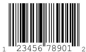
Figure 17.6: Code type: UPC-A
