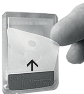
Figure 6.9: Attaching the diffusor foil
