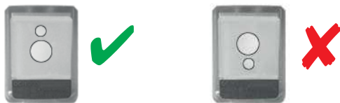
Figure 6.8: Orientation of the diffusor foil
