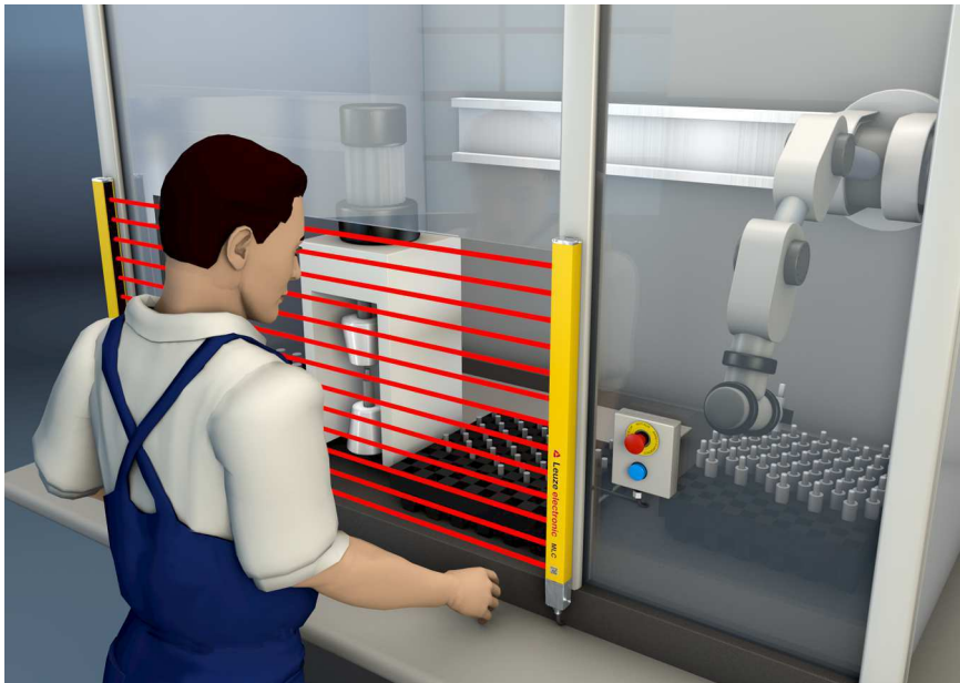
Fig. 5.2: Point of operation guarding protects reaching into the danger zone, e.g. for a pick & place robot application
