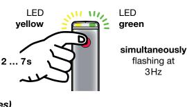
T ... 12s LED green alternatingly flashing at 3Hz
