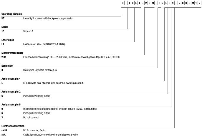
,200-M12 Cable, length 200 mm with M12 connector, 5-pin
