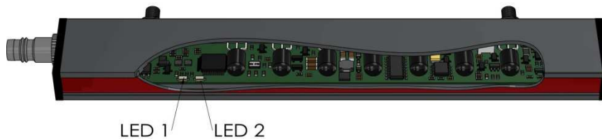
Figure 6: LED indicators/Error diagnostics
