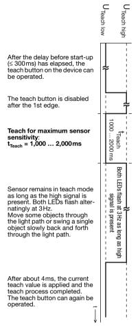
In the event of a teach error (e.g. no teach object or a teach object which is too small or too transparent is moved through the light path), the two LEDs flash at the same rate. Check the system, repeat the teach process, if necessary use a larger or less transparent teach object.
