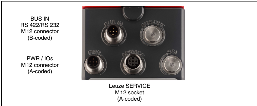
Figure 7.1: Connections of the AMS 300 i
