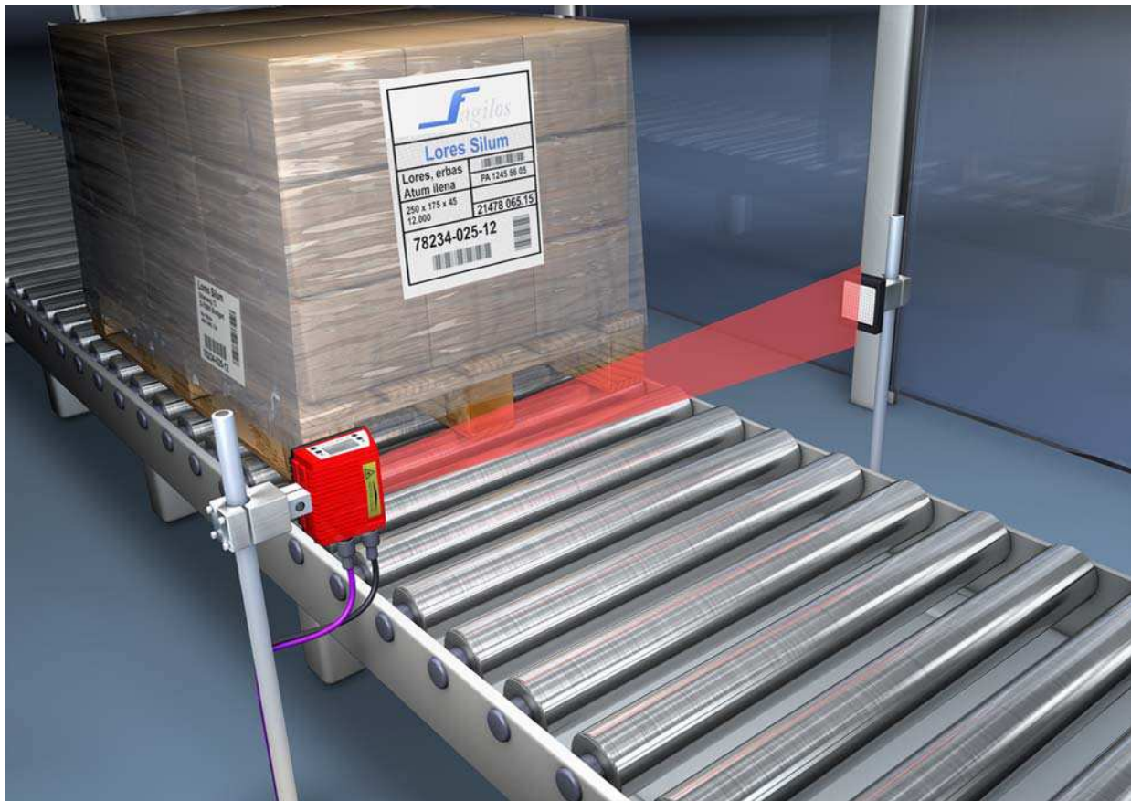
Figure 4.2: Reflector arrangement for autoReflAct
