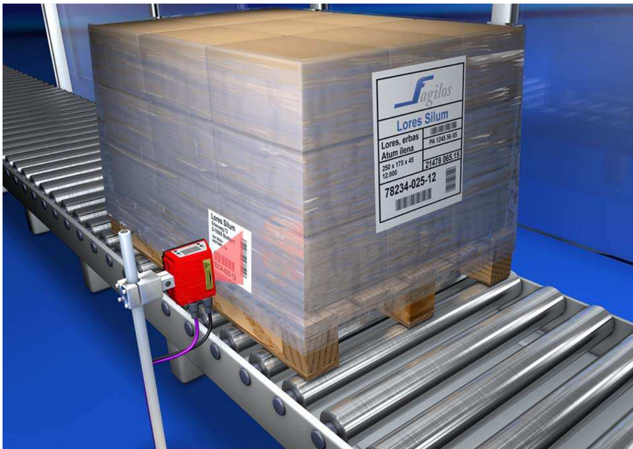
Figure 5.1: Deflection principle for the line scanner
