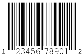
Figure 17.3: Code type 06: UPC-A
