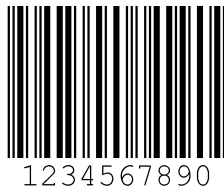
Figure 17.1: Code type 01: Interleaved 2 of 5
