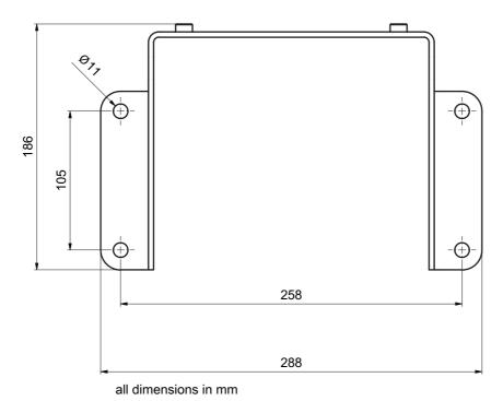
Figure 15.7: Mounting bracket BTF830M
