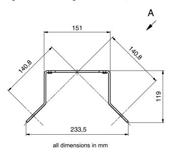
Figure 15.11: Mounting bracket BT856M
