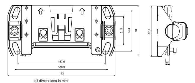
Figure 15.5: Mounting system BTU800M
