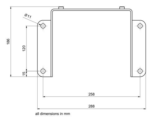
Figure 15.6: Mounting bracket BTF815M
