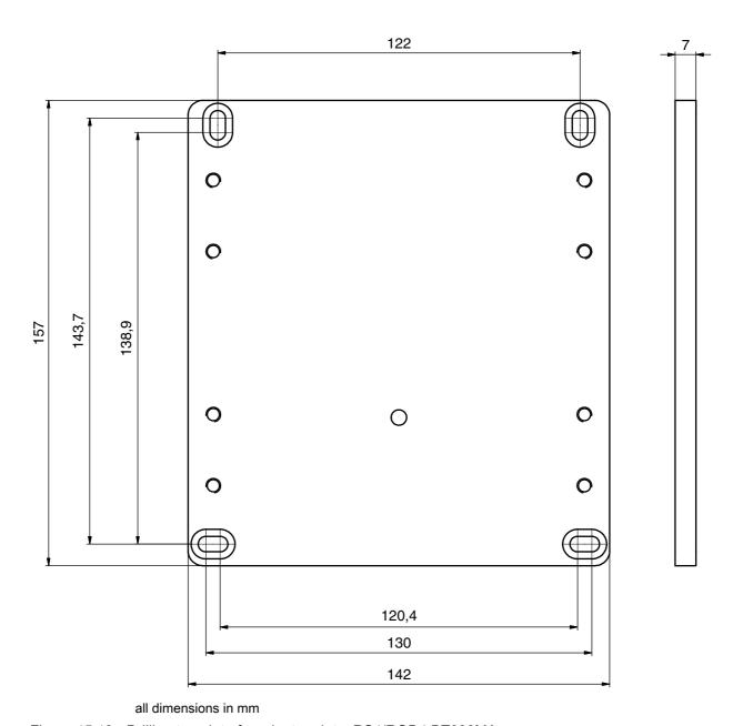
Figure 15.13: Drilling template for adapter plate, RS4/ROD4 BT800MA
