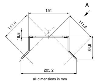
Figure 15.9: Mounting bracket BT840M
