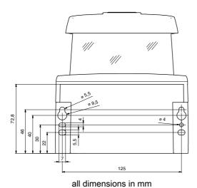
Figure 15.2: Mounting dimensions safety laser scanner with connection unit
