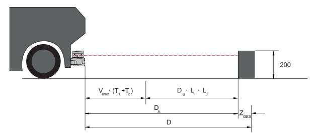
Figure 7.14: Mobile danger zone guarding, calculation of required minimum distance D
