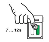
LED yellow LED green alternatingly flashing at 3Hz
