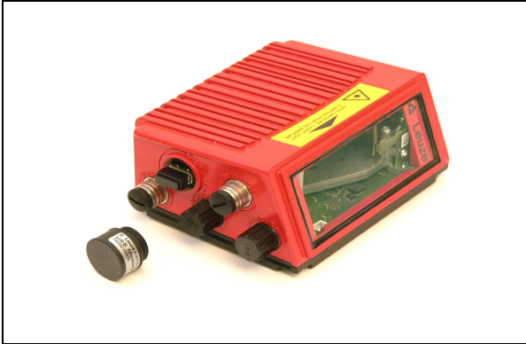
Figure 10.19: Installing the external parameter memory
