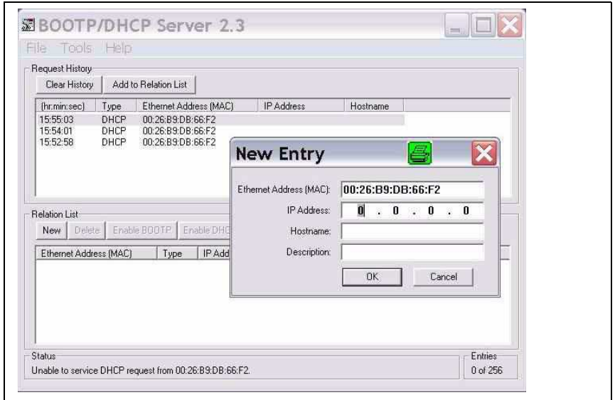
Figure 10.2: Manually setting the IP address
