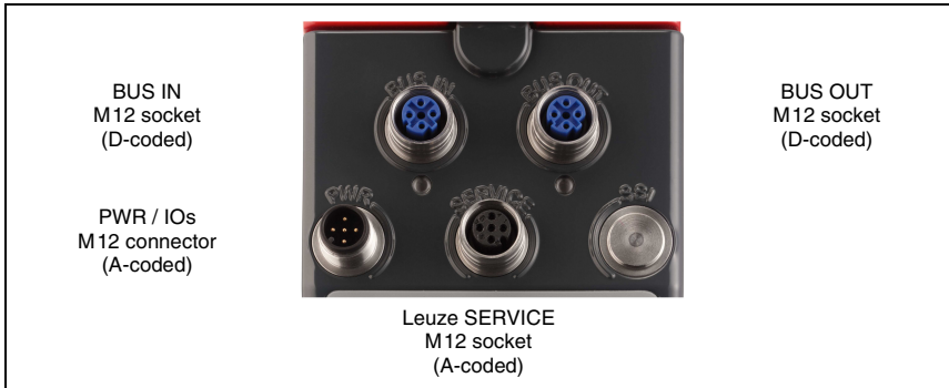
Figure 7.1: Connections of the AMS 338 i
