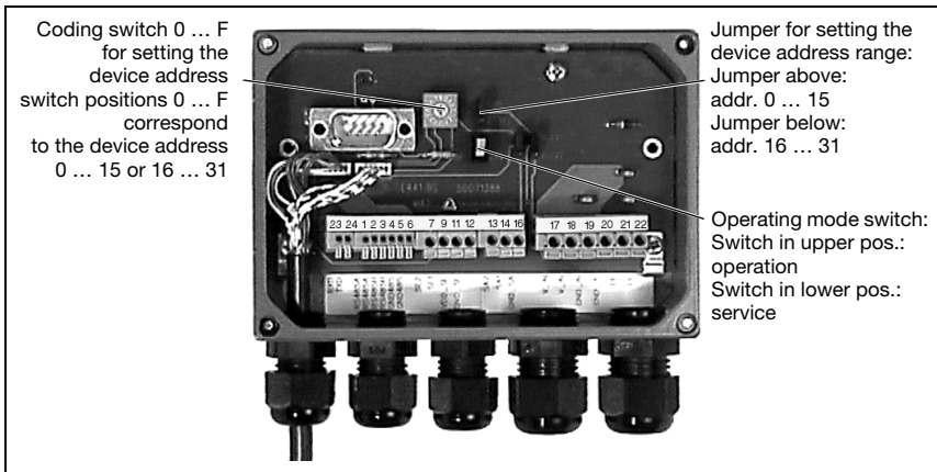
Figure 7.1: Configuration elements in the MA 2
