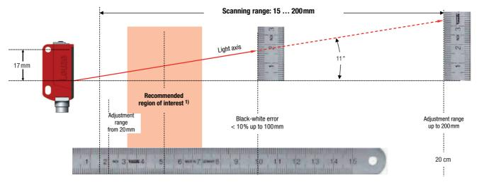
The ability of the sensor to reliably detect reflective surfaces or transparent objects is the strongest in the recommended working range. The sensor can also reliably detect such objects in the entire scanning range; however, the performance reserve is reduced in comparison to the recommended working range.
